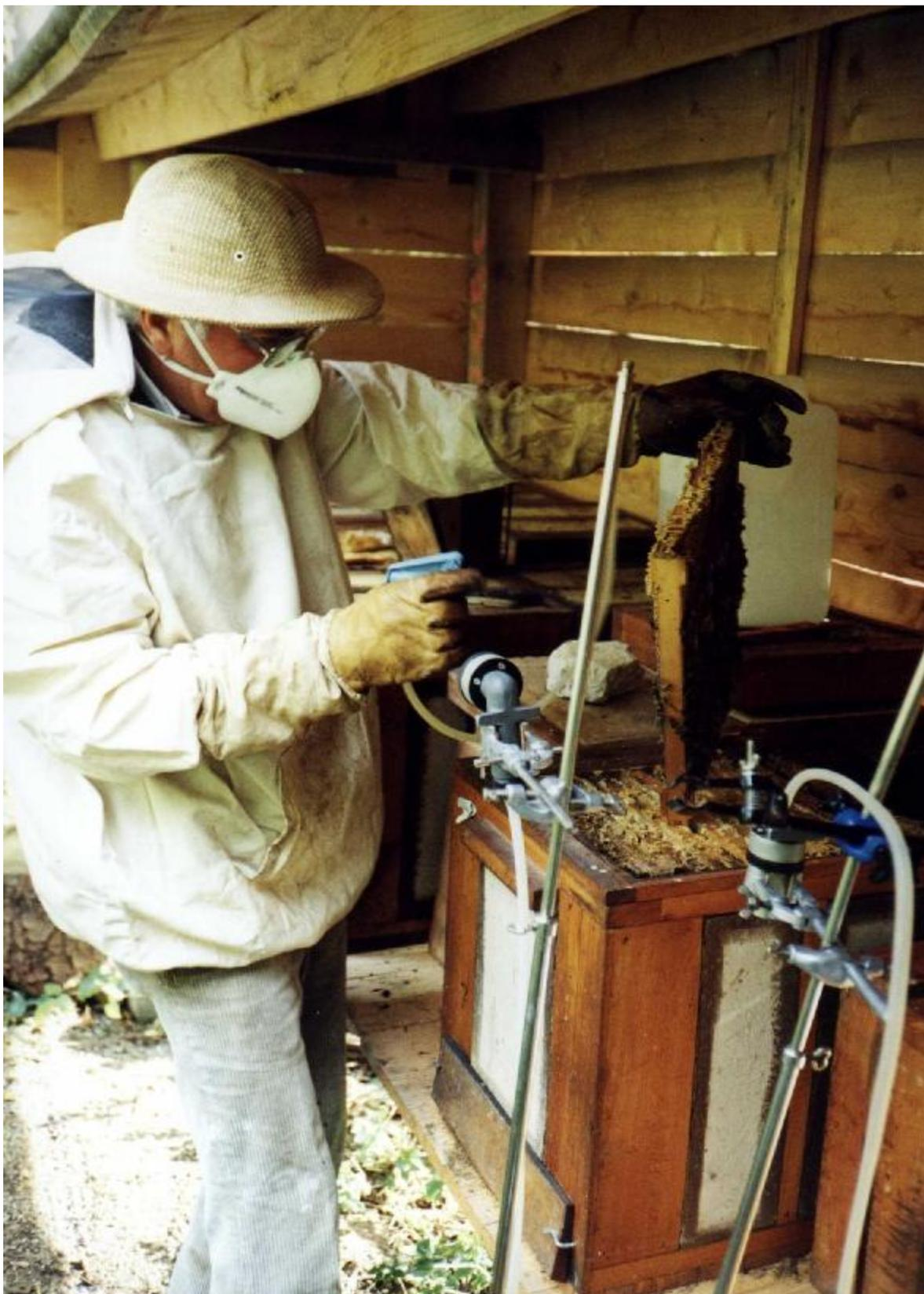
**Fig. 4:** Placing of the air sampler on a stand next to the beekeeper's working place. The beekeeper is spraying oxalic acid onto a honeycomb.
