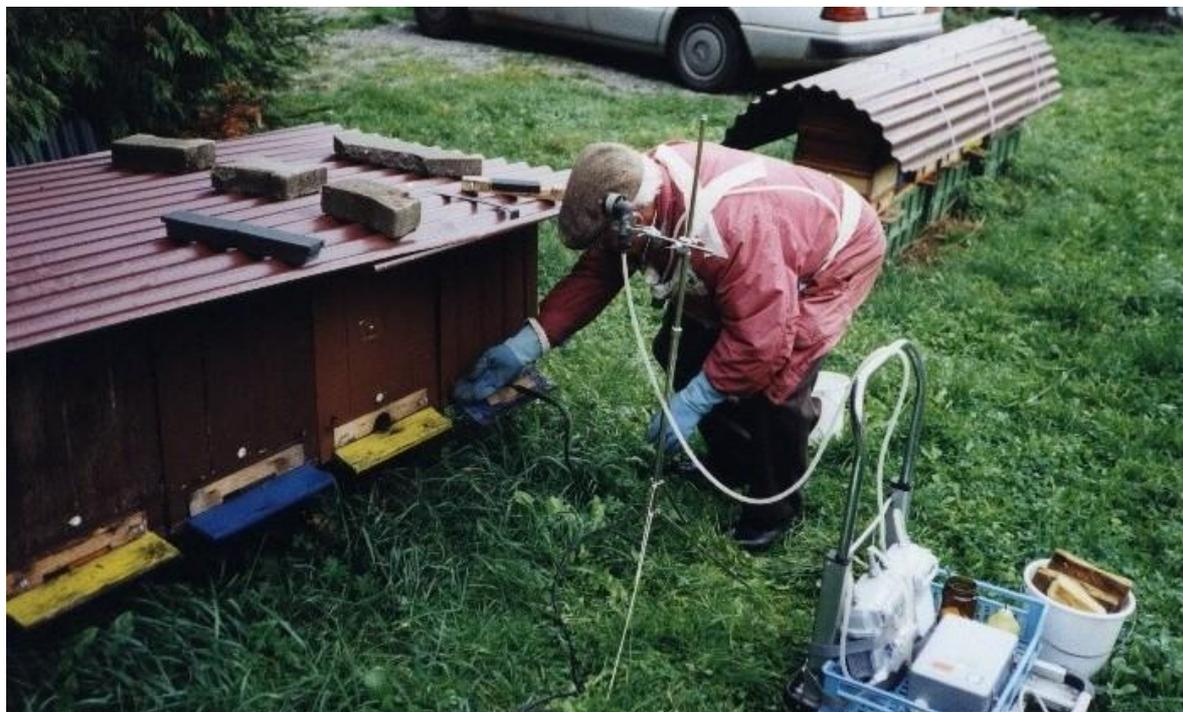
**Fig. 6:** The beekeeper is introducing the Varroa®-evaporator through the hive's entrance. In front of this the air sampler on a stand. On the right side the air collecting pump and the volume gauge.
