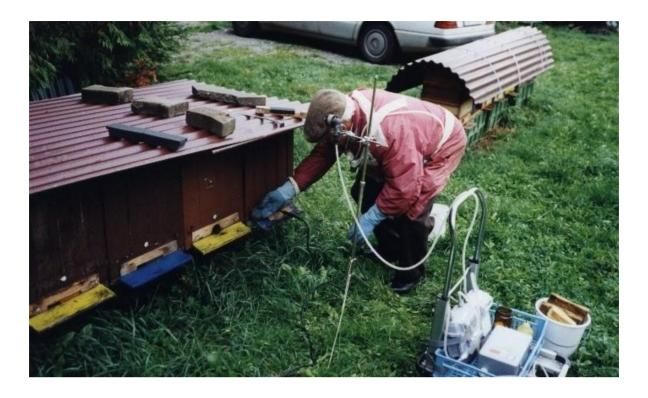
**Fig. 6:** The beekeeper is introducing the Varrox®-evaporator through the hive's entrance. In front of this the air sampler on a stand. On the right side the air collecting pump and the volume gauge.
