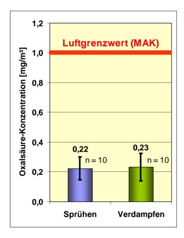
**Fig. 1:** Average values (and their confidence interval) of the measured oxalic acid concentrations in the air by both treatment methods. The number of independent measurements is indicated by "n". To direct comparison: The exposure-limit of oxalic acid is 1.0 mg/m<sup>3</sup>.
